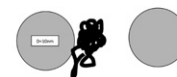
Simplified view of the relative size of a single polymer chain with R_g \approx 50 nm and particles with diameter 20 nm at 7 vol. % of the filler, when the average distance between regularly particles is about 2 particle diameters
